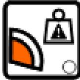
Light on indicates restricted range of motion due to platform weight.
