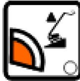
Light on indicates restricted range of motion due to platform weight and slope angle.
